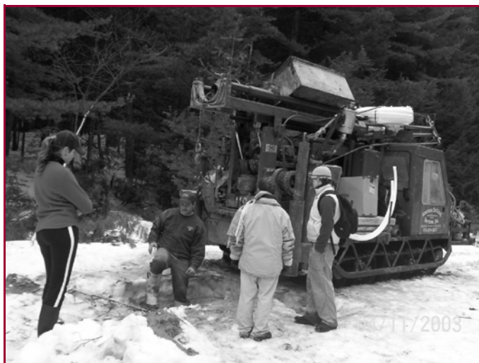
Drilling at Davis Mine. Preparing to drill a well into the tailings piles at the Davis Mine site last April. The driller has just excavated a hole in the snow to the ground surface and the rig will be raised into drilling position. From left to right are Mercedita Monserrate (M.S. student in Environmental Engineering), the driller, Melinda Solomon (student in School of Education), and Kate Berti (M.S. student in Geosciences).
